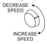
Figure 20. Throttle Control Switch
